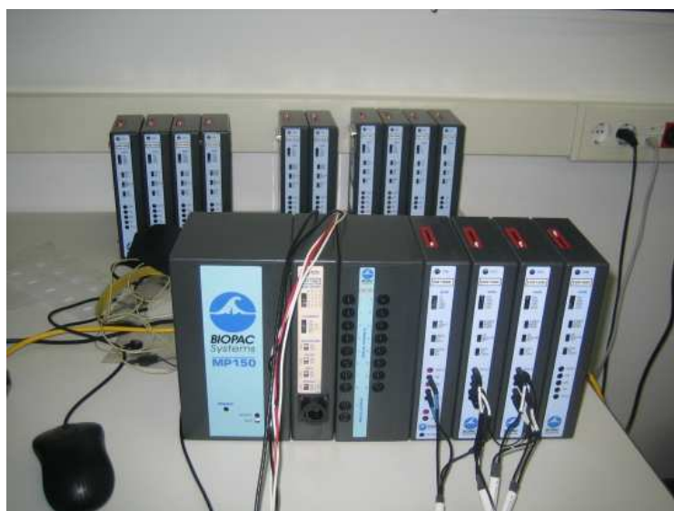
Fig. 2 MP150 System with electrodermal devices.
